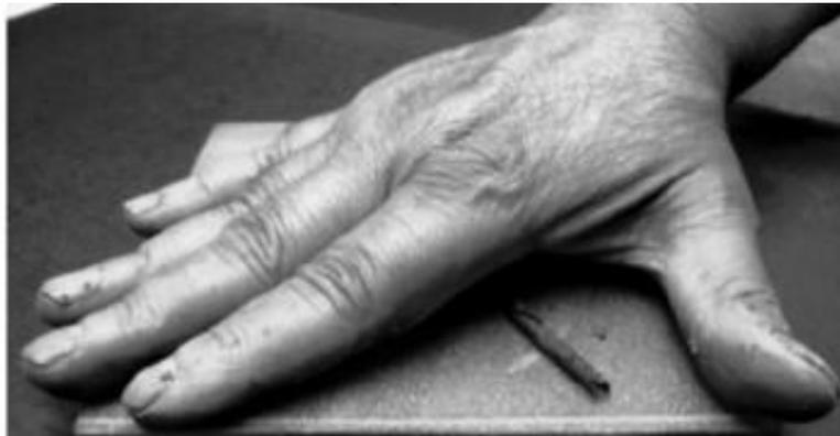
Figure (4) Rolling of soil mass on the ground glass plate to determine a plastic limit
