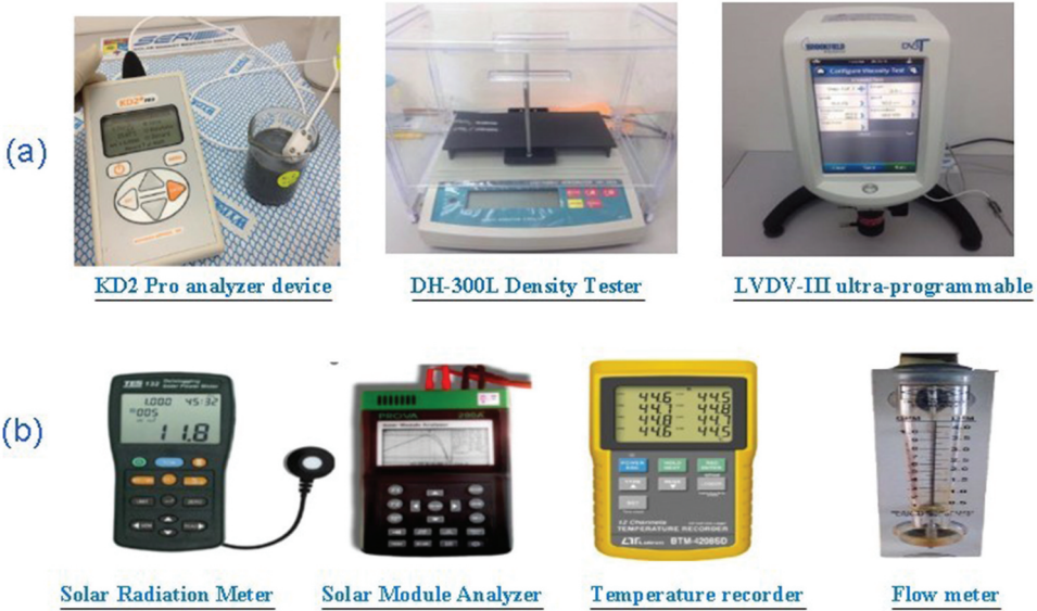
Figure 8. (a) Measurement devices for thermophysical properties, and (b) Measurement devices for experimental work.
