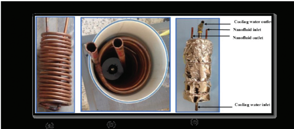
Figure 4. (a) Helical coil, (b) Coil inside shell, and (c) Assembled heat exchanger.
