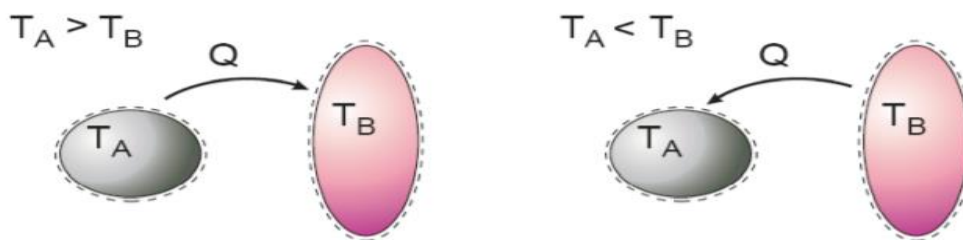
Fig. 9. Heat transfer occurs in the direction of higher-to-lower-temperature.
